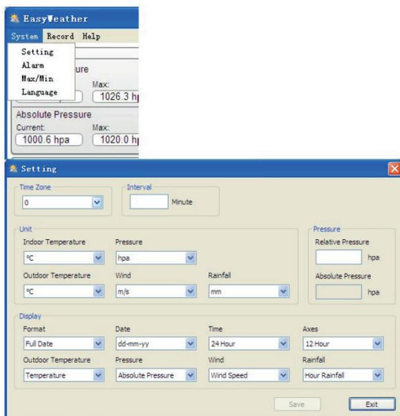
This section is used to set up PC software display, base station units, as well as able or disable the corresponding alarm function. Once you made your choice, press Save to make the setting effective.
