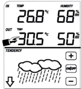
in great step. Touch the ON/OFF button to choose the alarm on or off (if alarm is enabled, the speaker icon will be turned on indicating the alarm function has been enabled).
