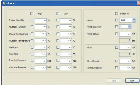
This section is used to set the desired time, high or low alarm value for the base unit. Once you made your choice, choose Save to make the setting effective. If you don't want to make any change, just press Cancel and exit without change.
