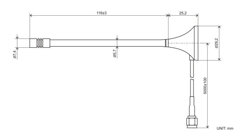
**VARIANTS** XAO-AGSM-MG2S Different connector variants or cable lengths are available on request.
