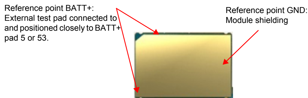
Figure 36: Position of reference points BATT+ and GND
