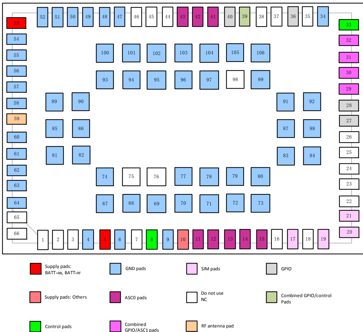
Figure 4: Numbering plan for connecting pads (bottom view)
