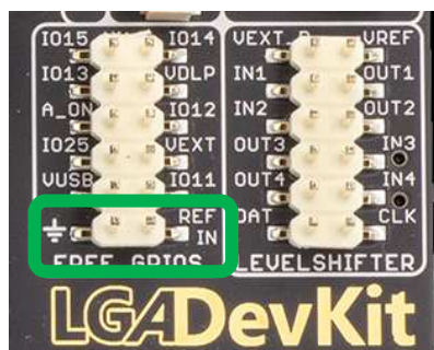
Picture: External reference supply and pin header for free level shifter
