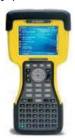
From 2007-2011, the Ranger X rugged handheld computer was purchased as a powerful tool for mobile workers around the world. The Ranger X computers featured an alphanumeric keypad, two user-accessible CompactFlash (CF) slots and one Secure Digital SD/SDIO slot for peripheral devices and additional storage. Embedded Bluetooth and 802.11 (wLAN) were optional features on some units.
