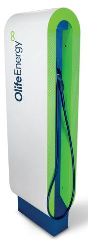
A fast charger (25 - 125 kW) for electric vehicles in a free-standing design case. Power electronics are mounted inside the charger chassis for power up to 75 kW. 100 kW and 125 kW stations need an external location for the power modules.
