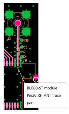
Figure 11: 50-Ohm trace design on BL600 development board (or host PCB) for use with BL600-ST module.
