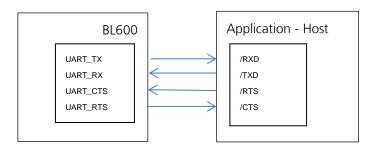
**Note:** The BL600 serial module output is at 3.3V CMOS logic levels (tracks VCC). Level conversion must be added to interface with an RS-232 level compliant interface.
