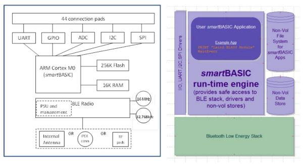
Figure 1: Functional HW and SW block Diagram for BL600 series BLE smartBASIC module
