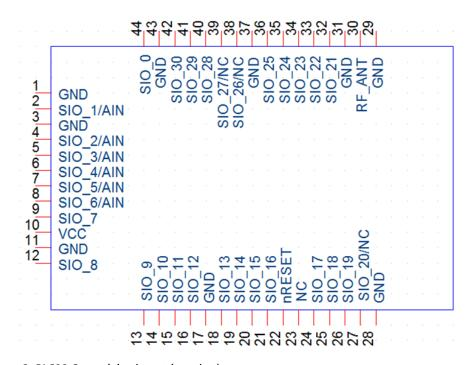
Figure 2: BL600-Sx module pin-out (top view).
