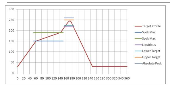
Figure 8-2: Recommended Reflow Temperature
