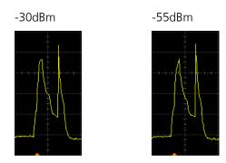
Figure 8: Typical peak current consumption profile during connection event in slave mode with TX Whisper mode TX PWR -30 dBm (TX Whisper Mode1) and -55 dBm (TX Whisper Mode2).
