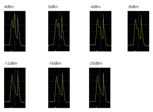
Figure 7: Typical peak current consumption profile during connection event in slave mode versus TX PWR.
