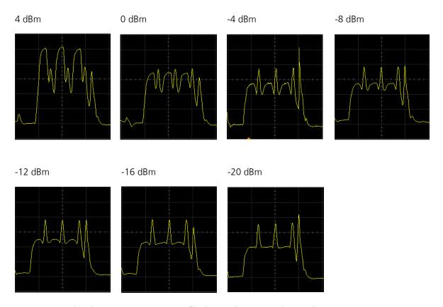
Figure 5: Typical peak current consumption profile during advertising in slave mode versus TX PWR
