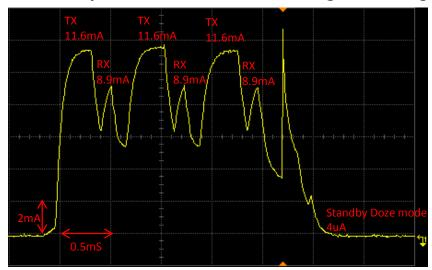
Figure 3: Typical peak current consumption profile during advertising in slave mode @ TX PWR +4dBm. UART is OFF. Last spike is DCDC being turned off.
